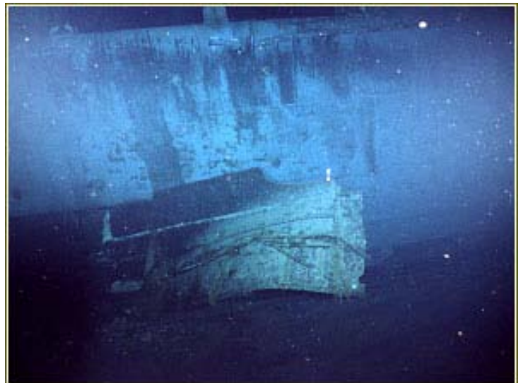
On the port side, a hole shows where two aerial torpedoes hit on June 4, 1942, ripping away armor plate and opening the hull. Oil stains above the hole indicate that the torpedoes ruptured fuel tanks
